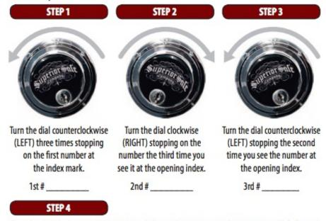
Turn the dial clockwise (right) until the dial completely stops at about 87. You will feel some resistance at about 97 but keep turning the dial until it completely stops. Then turn the safe handle clockwise to retract the locking bolts.
