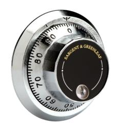
Sargent & Greenleaf mechanical locks consist of Three Combination Wheels, a Patented Sargent & Greenleaf Torque Adjuster, Integral Relock Trigger, and a Brass Four-Way Drive Cam. While other safe companies us lessadvanced locks, Sargent & Greenleaf locks have relockers, a feature that protects against drilling or torching. If a lock is tampered with, a relocker will lock up the last tumbler as an extra safety measure.
